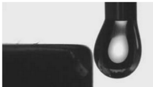
A droplet containing the soap is attracted to the magnet at left
