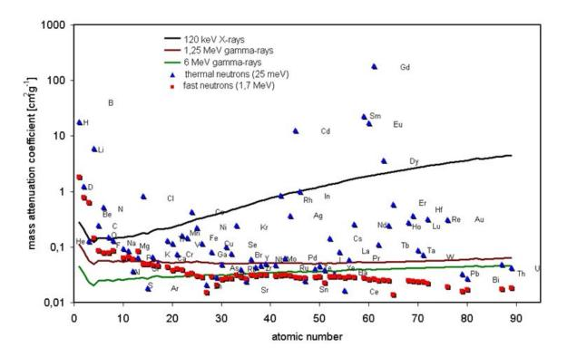
Mass attenuation coefficient for 125 keV X-rays, 1.25 MeV gamma rays, 6 MeV gamma rays, for thermal and for fast fission neutrons. While the cross section rises monotonously with atomic number, it decreases for fast fission neutrons, and shows no obvious regularity for thermal neutrons, often giving large contrast between neighboring atoms and isotopes.
