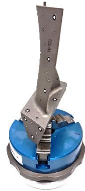
Sample mounted on robot holder
