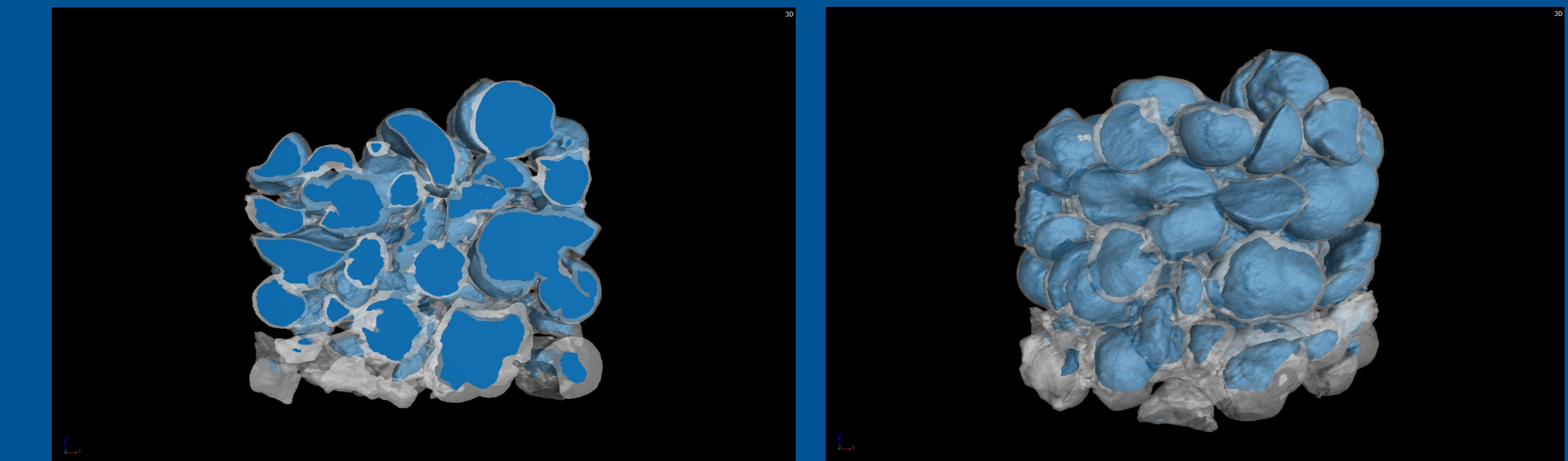
Fig. 6: Tomographic images of large particles showing ice in dark and dried material in light blue
