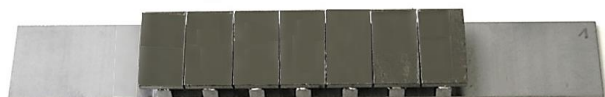
Fig. 7. A long HOPG crystal indium bonded on a ribbed silicon blade and then sliced into 9mm wide segments.
