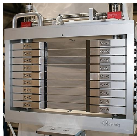
Fig. 9. Conventional double-focusing silicon monochromator with variable curvature composed of bent stacks of typically 10 perfect crystals each. (Courtesy: Positechnics).
