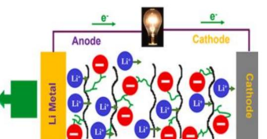
Two electrode along with electrolyte embedded in between.
