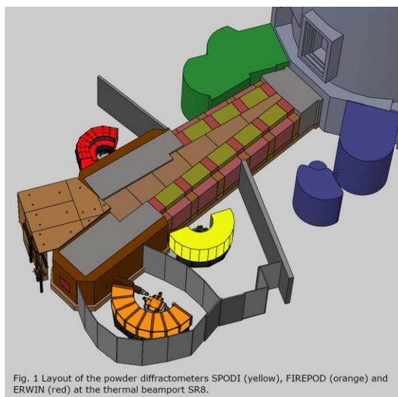
Fig. 1 Layout of the powder diffractometers SPODI (yellow), FIREPOD (orange) and ERWIN (red) at the thermal beamport SR8.
