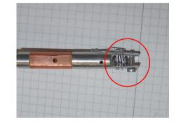
High quality single crystal of HoFeO<sub>3</sub>, dimensions 5x6x7 mm<sup>3</sup>. Neutron diffraction experiments were performed at MLZ on two axes single crystal diffractometer POLI using a new 8T magnet. Crystal was slowly cooling in the magnet with zero
