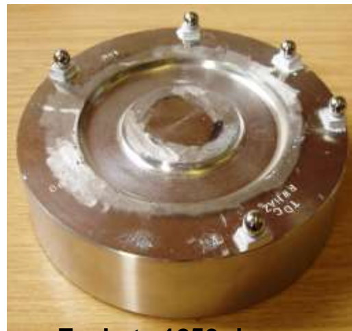
Esshete 1250 ring-welds(HAZ and repair designs)
