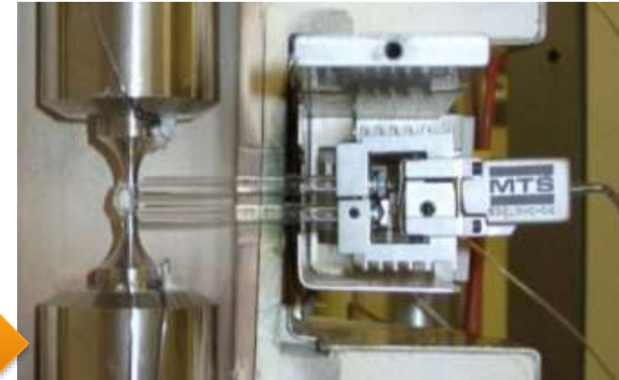
Conventional isothermal tensile and cyclic tests
