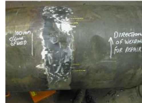
316H SS, 35mm pipe butt weld and with 218mm offset repair
