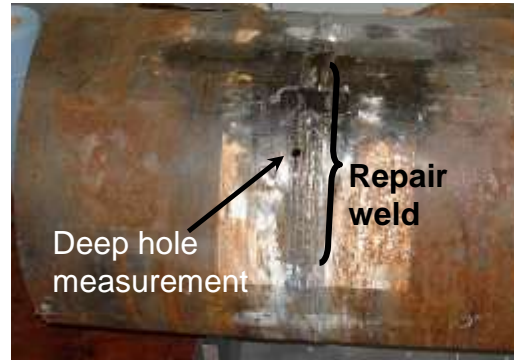
316H SS 19.6mm pipe butt weld & with short & long repairs
