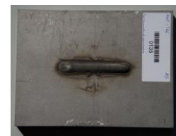
TG6 mock-up : Welding + Grinding [2]
