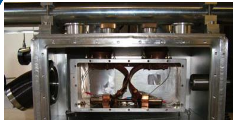
(1) two Leybold 1245 CCRs; (2) an outer vacuum vessel with aluminium windows to provide access for the incident and scattered neutrons; (3) the infrared radiation shield which is connected by thermal links (7) to the first stages of the CCRs; (4) the thermal links connecting the CCR second stages to the rig jaws; (5) the test sample; and (6) the 50 kN hydraulic stress rig.
