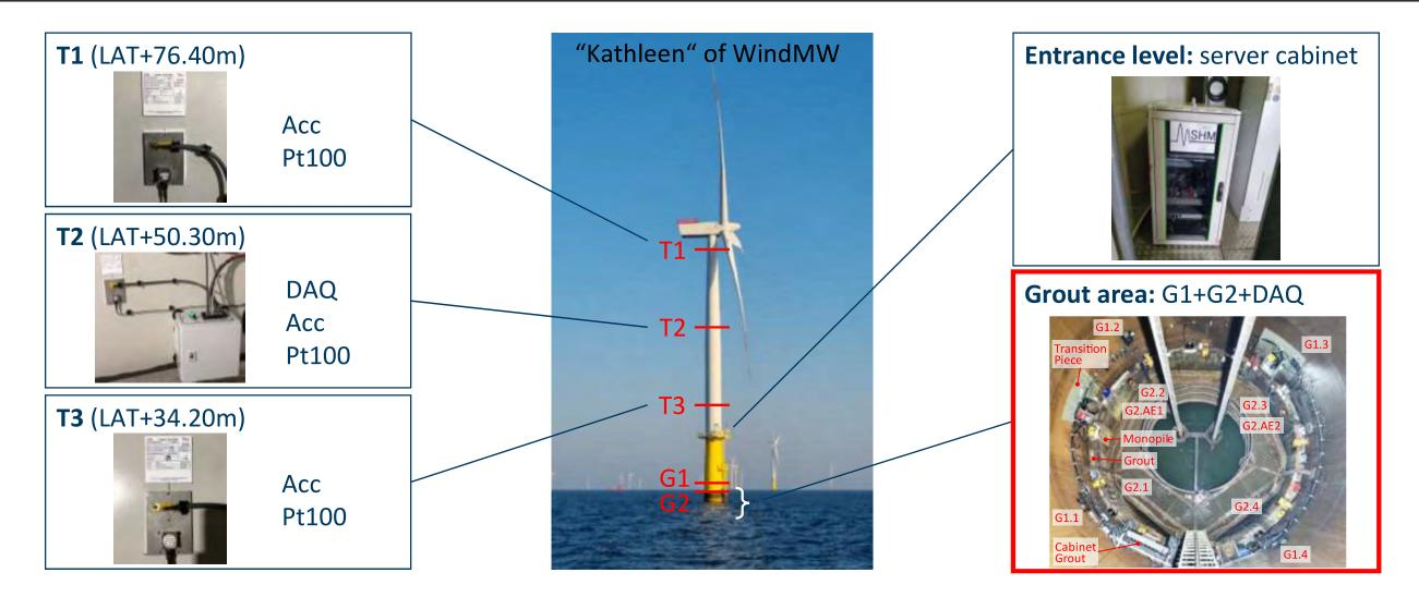
Offshore installation of 100 measurement channels and the entire measurement system was completed in **just 5 days by** Fraunhofer LBF and University of Siegen!
