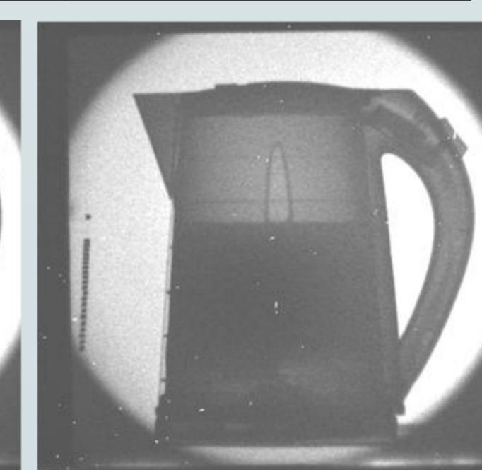
Fig. 10- Image for kettle captured from {}^6\text{LiF-ZnS} , produced by neutrons, EM=200, AET = 9.94 s, Bi in beam, Cd and Boral out of beam.
