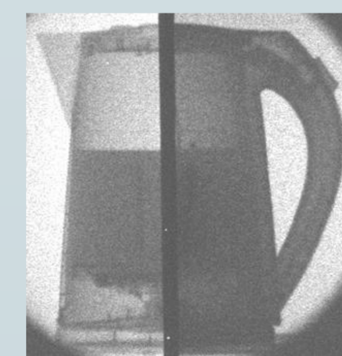
Fig. 11- Image for kettle captured simultaneously on Lanex (left part, with neutrons and gammas) and {}^6\text{LiF-ZnS} (right part, with neutrons) from a video, EM=255, AET = 0.9 s, Bi, Cd and Boral out of beam, before water boiling.
