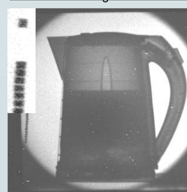
Fig. 7- Image for kettle captured from {}^6\text{LiF-ZnS} , produced by neutrons, EM=180, AET = 9.76 s, Bi, Cd and Boral out of beam.
