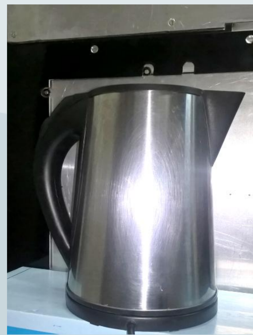
Fig. 2 – An electrical water kettle put in front of the scintillator's aluminum holder on rotary table.
