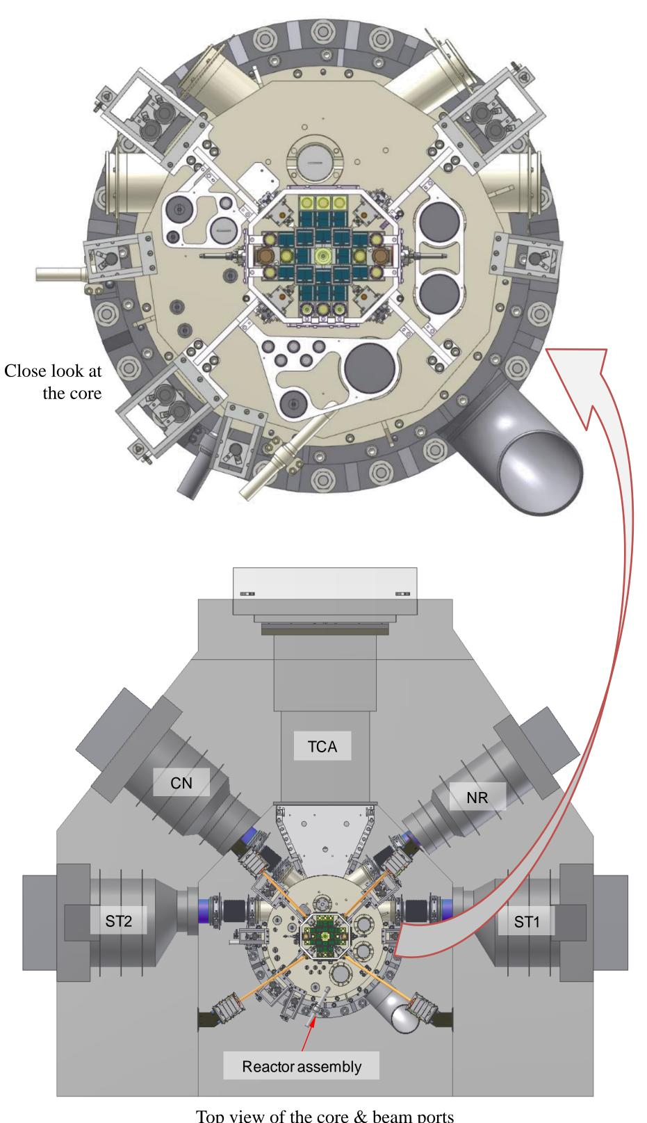
Top view of the core & beam ports
