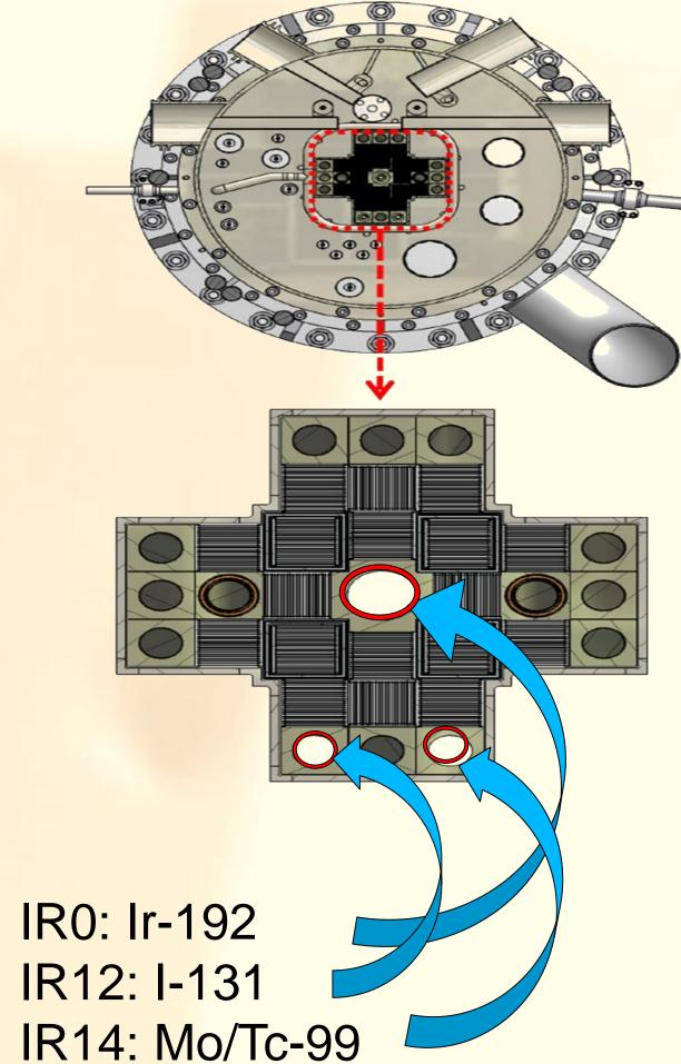
Other locations in the core can be used for future RI production (with various irradiation times).
