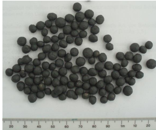
Steel granulate with a layer of wax and boron powder
