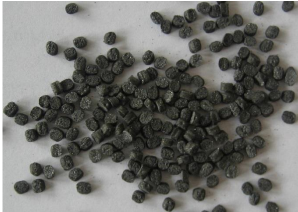
Polyethylene pellets with boron and iron powder
