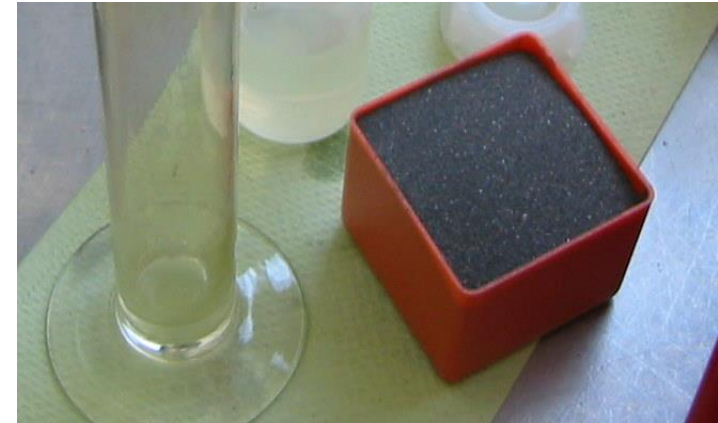
A mixture of iron powder, ferroboron powder and liquid paraffin
