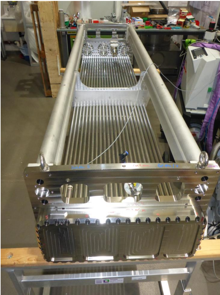
Module with 23 tubes on test bench in lab
