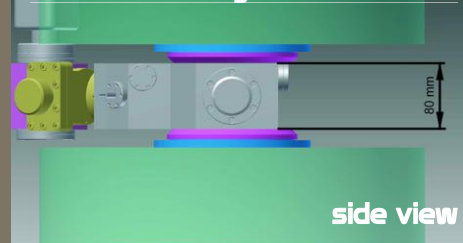
Proposed PLD setup concept for in vacuo investigations @ MARIA
