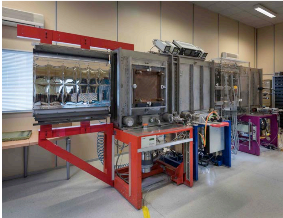
Sputtering machine (ILL) - Production 0.8 m 2 / day
